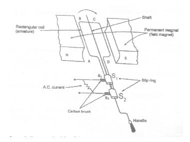
After every half revolution, each side of the generator coil starts moving in the opposite direction in the magnetic field. The side of the coil which was initially moving upwards, after half revolution, it starts moving downwards. Due to the change in the direction of motion of the two sided of the coil in the magnetic field every half revolution, the direction of current produced in them also changes after every half revolution.
