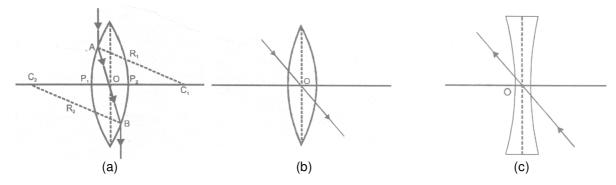
Figure: Ray diavram Showing lateral displacement
