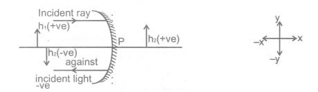
Focal length concave mirrro is -ve Focal length of convex mirror is +ve
