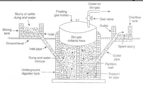
Floationg gas holder type biogas plant
