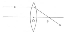
Figure: Convex Lens
