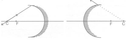
Concave Convex (iii) A ray incident through the focus is reflected parallel to the principal axis.
