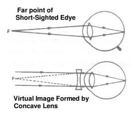
Note that focal length of the lens for a short-sighted person is equal to the negative value of the person's far point.
