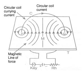
Direction of magnetic field is found by applying the right hand thumb rule to each section of the coil and we find that the concentric lines of force pass through the coil in the same direction. Further more that:
