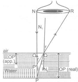
In above fig.  $\angle PQN_2 = \angle i \& \angle N_1OR = \angle r$
