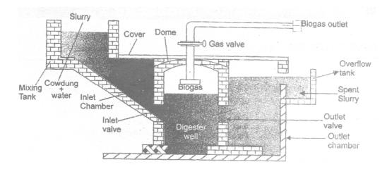
**Fixed Dome Type Biogas Plant**
