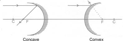
(ii) A ray incident through the centre of curvature (C) falls normally and is reflected back along the same path.
