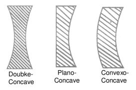
Figure : Different types of concave lens
