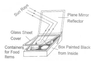
Solar cooker is a device used for cooking food with the help of solar energy. A box is made of a non - conducting material like plastic or fiber glass and painted black from inside is used for making the solar cooker.
