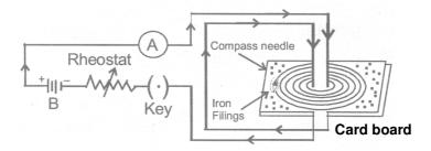
The magnetic lines of force form concentric circles near the wire, with their plane perpendicular to the straight conductor and with their centers lying on its axis. if the direction of current in the wire is reversed, the direction of lines of force is also reversed.
