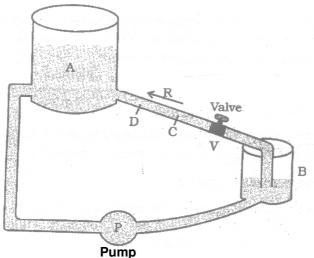
In the same manner electrons will move along a wire only if there is a difference of electric pressure called potential difference along the conductor. This difference of potential produced by the cell or a battery, which acts like a water pump in the circuit.
