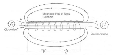
The magnetic field, thus produced, is very much similar to that of a bar magnet and one end of the coil acts like a magnetic north pole while the other acts like a south pole.
