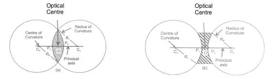
Figure: Characteristics of convex and concave lenses
