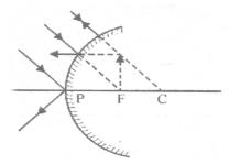
(ii) When the object is placed between infinity and the pole then the image is formed between the focus and the pole. The image formed is virtual, erect and diminished.
