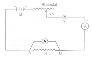
Note the successive readings in the ammeter and the voltmeter. WE will find that with two cells in the circuit, the current would be **2I** and the potential difference **2v**. Similarly, with three cells the current is **3I** and potential difference **3v** and so on. [The important precaution to observe here is not allow the current of flow in the wire continuously. This can be done by taking off the plug key and closing it only when the current is to be drawn.]
