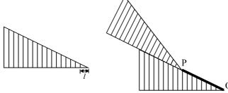
In this diagram, we are interested in measuring the length of the line PQ. If the angle of both the inclines is equal to  $\theta$  then what is the least count of the instrument.
