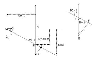
In this method we watch the velocity of A w.r.t. D. To do the accelerations of both the bodies is zero, so the relative acceleration between them is also zero. Hence the relative velocity will remain constant. So the path of A with respect to B will be straight line and along the direction of relative velocity of A with respect to B. The shortest distance between A & B is when A is at point of the when we drop a perpendicular from B on the line of motion of A with respect to B).
