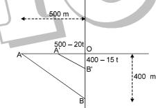
A & B be are the initial positions and A',B' be the final positions after time t. B is moving with a speed of 15 m/sec so it will travel a distance of BB' = 15t during time t. A is moving with a speed of 20 m/sec so it will travel a distance of AA' = 20t during time t. So
