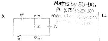
In the circuit shown, the current in the  $1\Omega$ resistor is :
